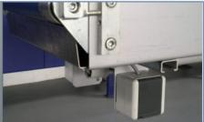
Leftovers are scraped off automatically at the end of the conveyor and collected into a removeable drawer.
